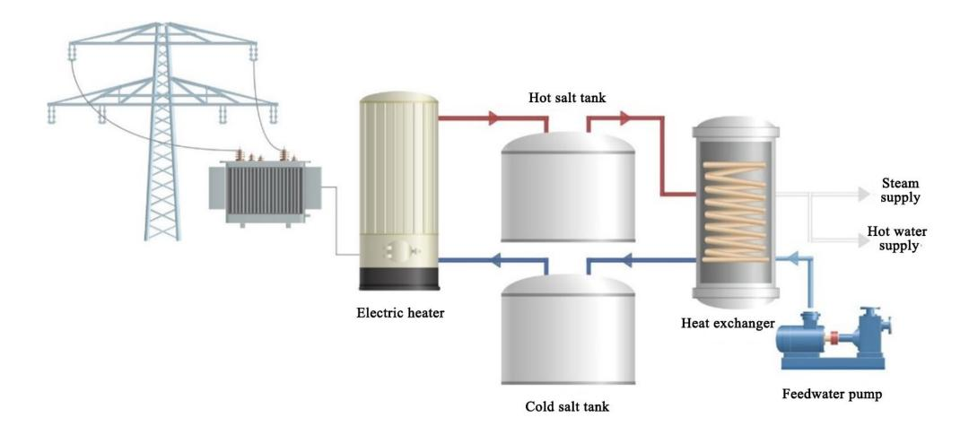
The molten salt is used to store energy at low temperature and release energy at high temperature for off-peak use.
