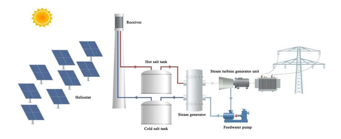
The heliostat gathers the sunlight and heats the molten salt to generate high-temperature and high-pressure steam to drive the steam turbine generator unit for power generation.
